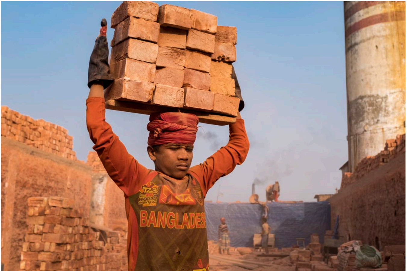
BRICK PRODUCTION ON THE OUTSKIRTS OF DHAKA, BANGLADESH, FALLS TO SEASONAL WORKERS AND CAN BE DONE ONLY IN THE DRY WINTER SEASON. WORKERS, CLOCKWISE FROM TOP LEFT ON OPPOSITE PAGE, LINE UP RAW BRICKS TO DRY BEFORE FIRING, CARRY FIRED BRICKS TO TRANSPORT TRUCKS, STACK FIRED BRICKS, TAKE BUCKETS OF COAL POWDER TO KILNS FOR FUEL, SEPARATE FIRED BRICKS, AND REMOVE FIRED BRICKS FROM A KILN.
