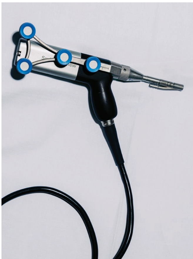
DURING KNEE REPLACEMENTS, THIS CUTTING TOOL PROVIDES SURGEONS WITH HAPTIC FEEDBACK TO KEEP THEIR BONE RESECTIONS WITHIN BOUNDS ESTABLISHED BY A 3D MODEL. THE BLUE DISCS ARE LOCATION TRACKERS.
